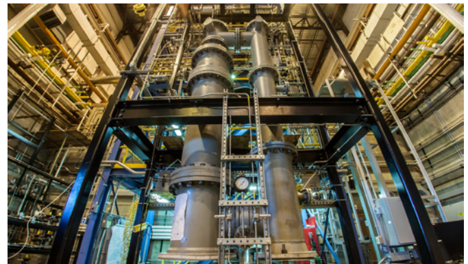
The Chemical Looping Reactor at NETL, Morgantown, West Virginia – The combustion of fossil fuels in nearly pure oxygen, rather than air, presents an opportunity to simplify CO 2 capture in power plant applications. Chemical looping combustion is considered a potentially “transformational” technology.
